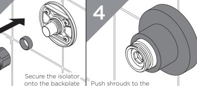
Push shrouds to the back of the wall outlet. securing them against the gasket.
